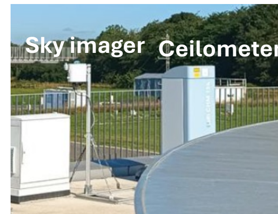
Example of dual ground-based sensor setup for solar forecasting
